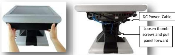
4. Unclip the retaining clamp to access the cables.
