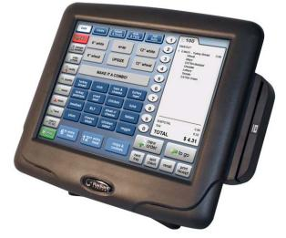
This package includes a 15" active matrix, color, 1024X768 main display with a resistive touch screen. The 15" display is a *56% increase* in surface area over the 12" models which allows for faster transactions due to less toggling between application screens, more application design flexibility, and better resolution. The bright active matrix screen provides the best possible display quality, with excellent contrast and brightness.
